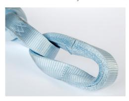
If stitching is torn/abraded, and there is a risk the layers of webbing can unravel, the chain must be removed from service immediately and should be discarded.
