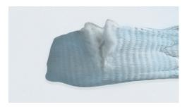
If there are visible cuts or abrasion of more than 1 mm on the side of the link leg, Green Pin Tycan® Lifting Chain must be removed from service immediately and should be discarded.
